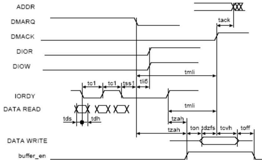
Figure 16. UDMA In Device Terminates Transfer Timing Diagram
