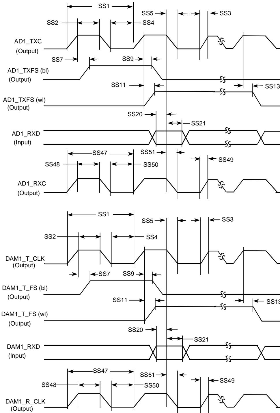
Figure 81. SSI Receiver with Internal Clock Timing Diagram
