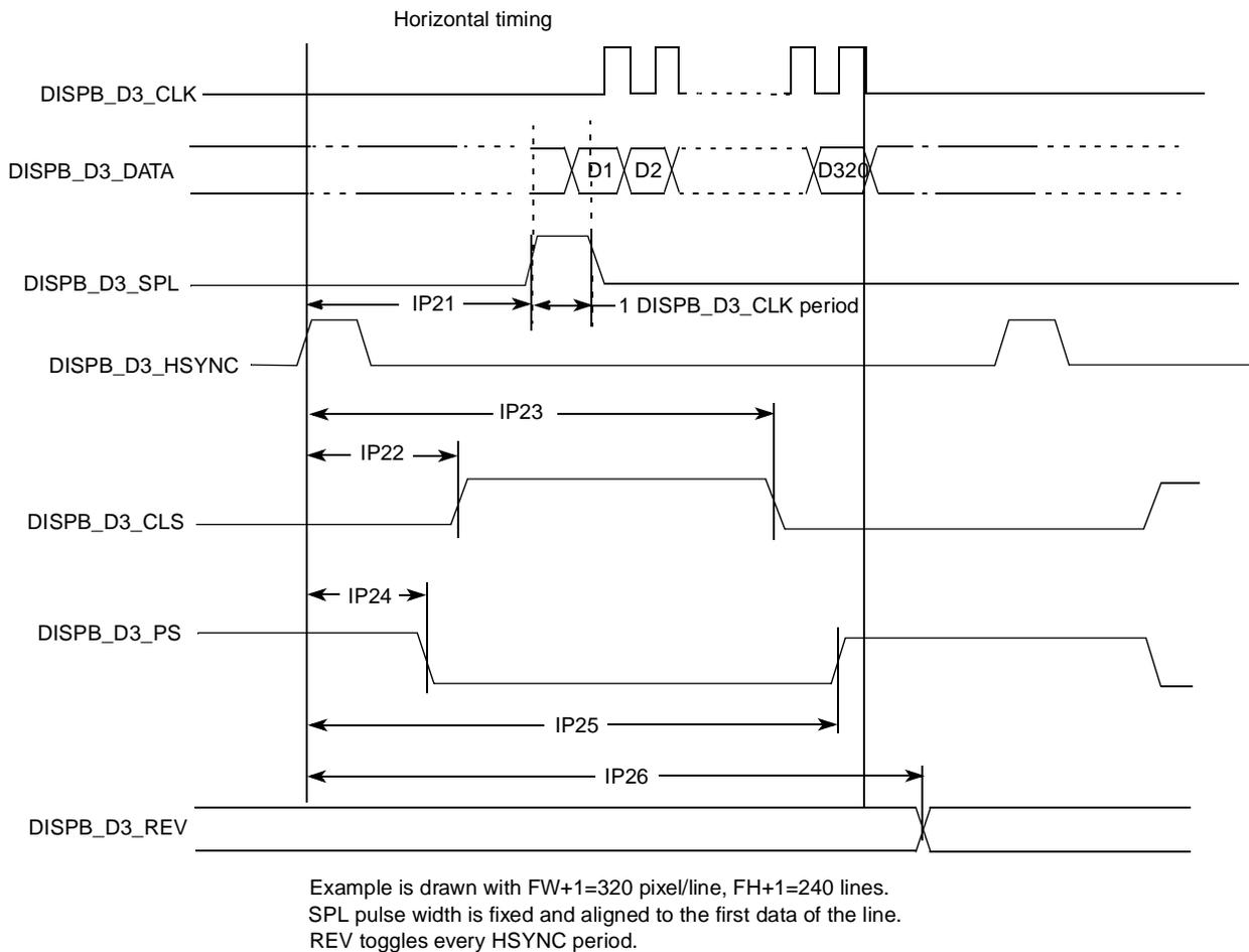
**Figure 49. Sharp HR-TFT Panel Interface Timing Diagram—Pixel Level**
