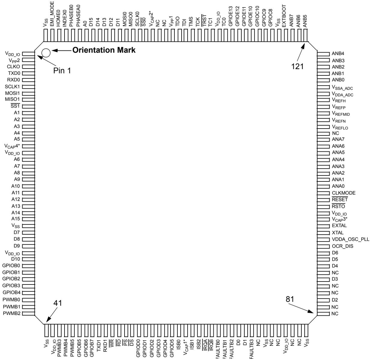
\* When the on-chip regulator is disabled, these four pins become 2.5V V<sub>DD\_CORE</sub>.
