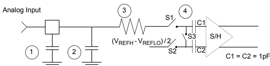
1. Parasitic capacitance due to package, pin-to-pin and pin-to-package base coupling; 1.8pf
