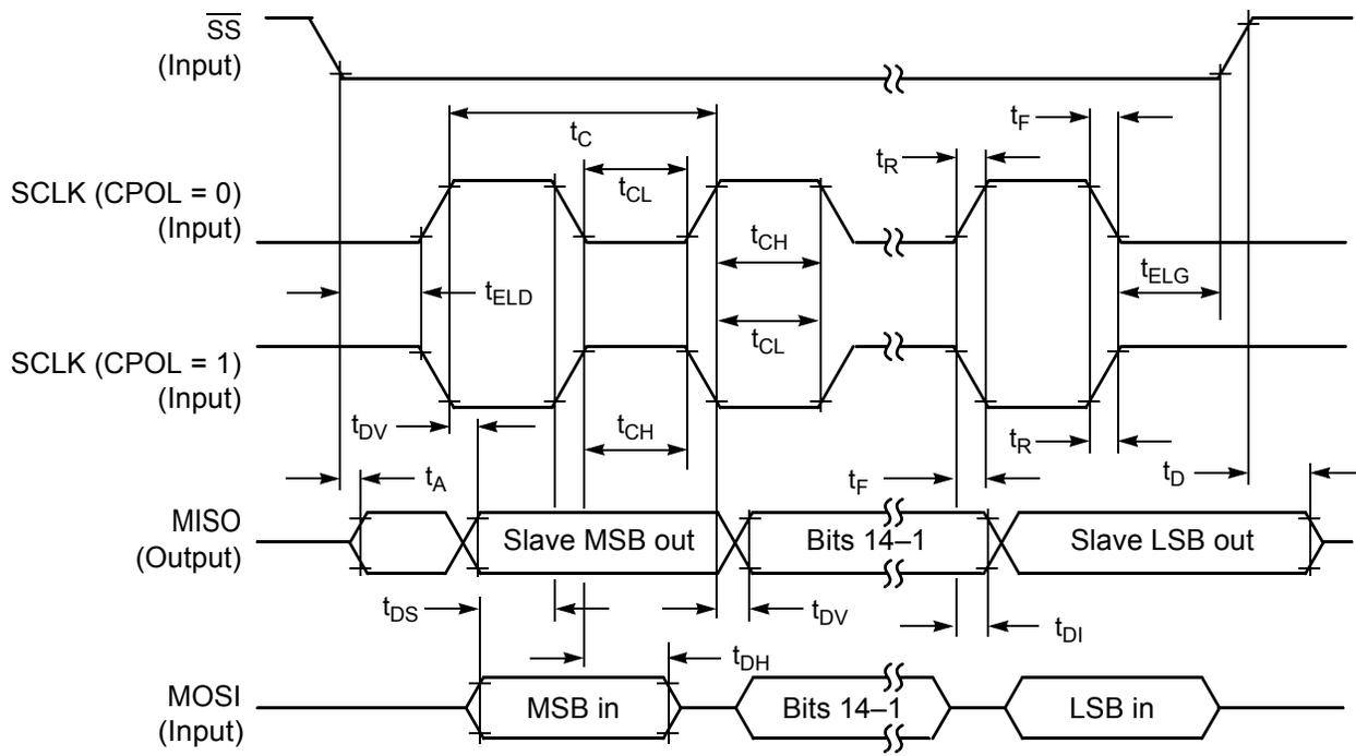
**Figure 10-13 SPI Slave Timing (CPHA = 1)**
