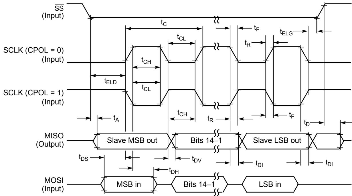
**Figure 10-12 SPI Slave Timing (CPHA = 0)**
