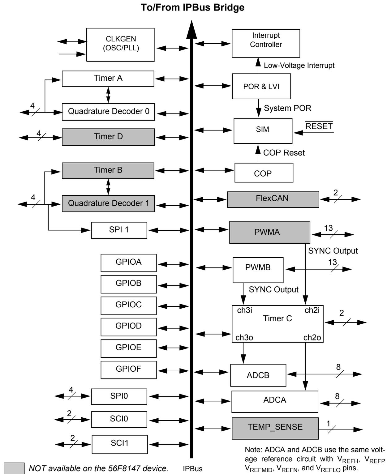
**Figure 1-2 Peripheral Subsystem**
