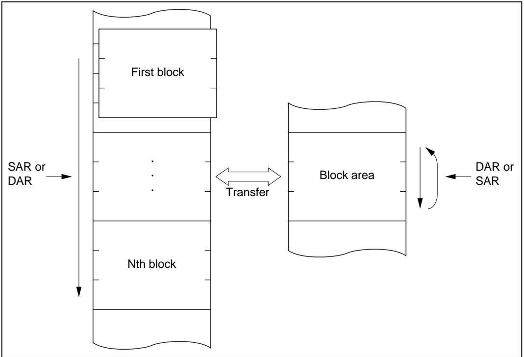
**Figure 8.8 Memory Mapping in Block Transfer Mode**
