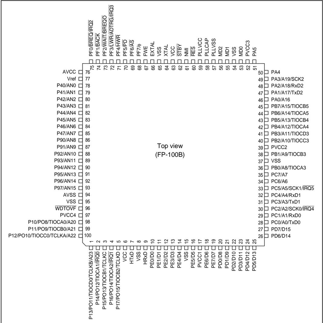
Figure 1.3 Pin Arrangement (FP-100B: Top View) (H8S/2623 Group)
