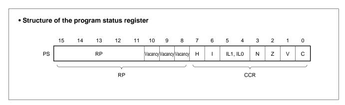
The RP indicates the address of the register bank currently in use. The relationship between the pointer contents and the actual address is based on the conversion rule illustrated below.
