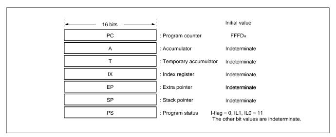
The PS can further be divided into higher 8 bits for use as a register bank pointer (RP) and the lower 8 bits for use as a condition code register (CCR). (See the diagram below.)
