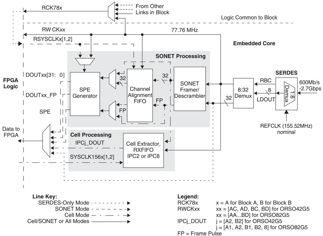
In either the SONET or cell mode, data from the DEMUX is then passed through a framer which word aligns and frames the data. Data are then processed based on cell mode or SONET mode selection.
