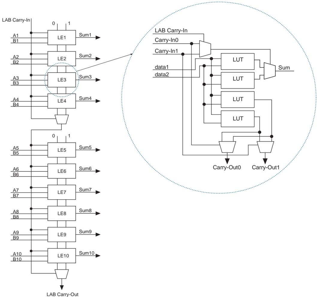
The Quartus II Compiler can create CSLA logic automatically during design processing. Alternatively, the designer can create CSLA logic manually during design entry. Parameterized functions such as library of parameterized modules (LPM) and DesignWare functions automatically take advantage of carry chains for the appropriate functions.
