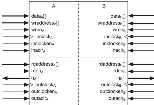
In addition to quad port memory, the ESB also supports true dual-port, dual-port, and single-port RAM. True dual-port RAM supports any combination of two port operations: two reads, two writes, or one read and one write. Dual-port memory supports a simultaneous read and write. For single-port memory, independent read and write is supported. [Figure 18](#) shows these different RAM memory port configurations for an ESB.
