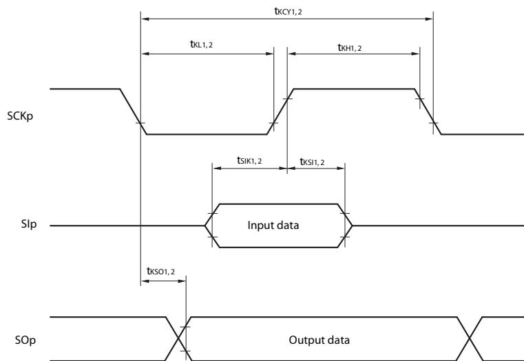
**CSI mode serial transfer timing (during communication at same potential)**(When  $\text{DAPmn} = 0$  and  $\text{CKPmn} = 1$ , or  $\text{DAPmn} = 1$  and  $\text{CKPmn} = 0$ .)
