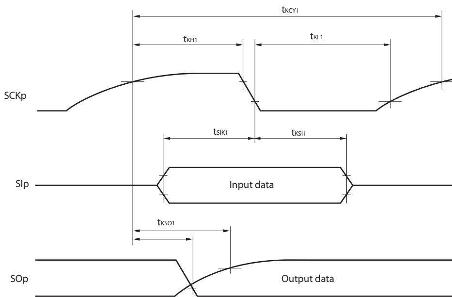
(9) Communication at different potential (1.8 V, 2.5 V, 3 V) (CSI mode) (slave mode, SCKp... external clock input)
