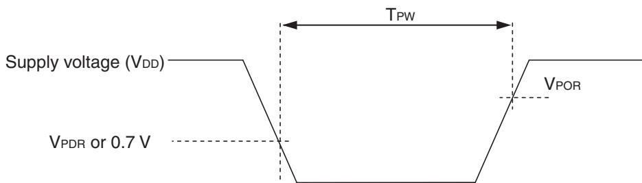
**LVD detection voltage of interrupt & reset mode**(T<sub>A</sub> = -40 to +105°C, V<sub>PDR</sub> ≤ V<sub>DD</sub> ≤ 5.5 V, V<sub>SS</sub> = 0 V)
