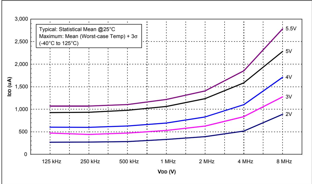
**FIGURE 20-13: TYPICAL I<sub>PD</sub> vs. V<sub>DD</sub> (SLEEP MODE, ALL PERIPHERALS DISABLED)**
