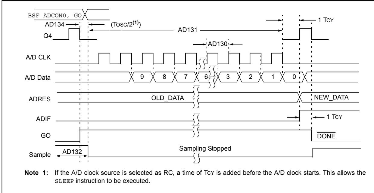
**FIGURE 19-10: PIC16F913/914/916/917/946 A/D CONVERSION TIMING (SLEEP MODE)**
