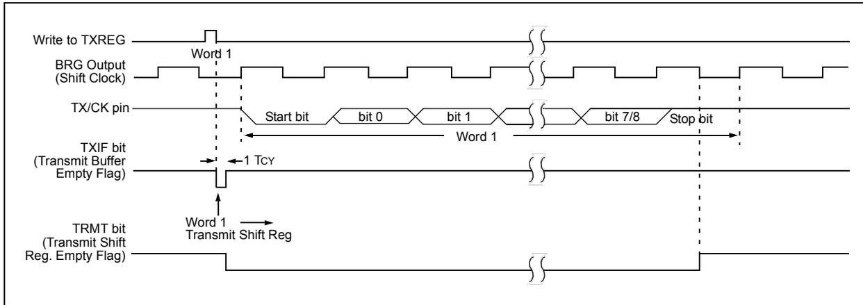
**FIGURE 9-4: ASYNCHRONOUS TRANSMISSION (BACK-TO-BACK)**
