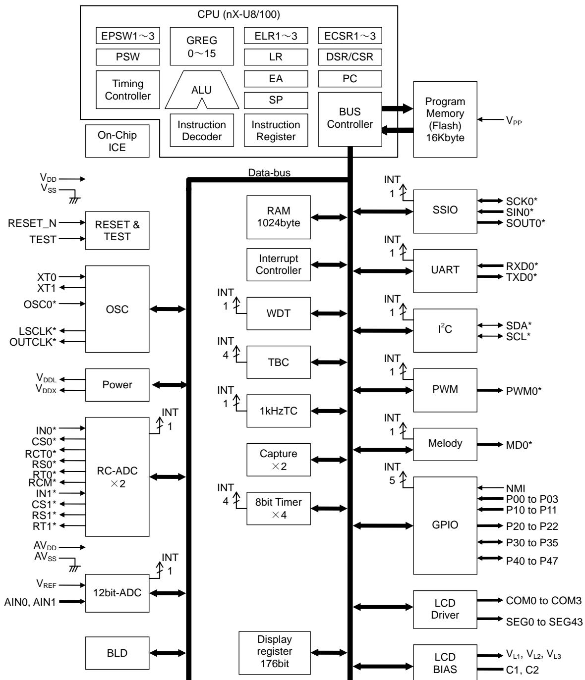
Figure 2 ML610Q412 Block Diagram
