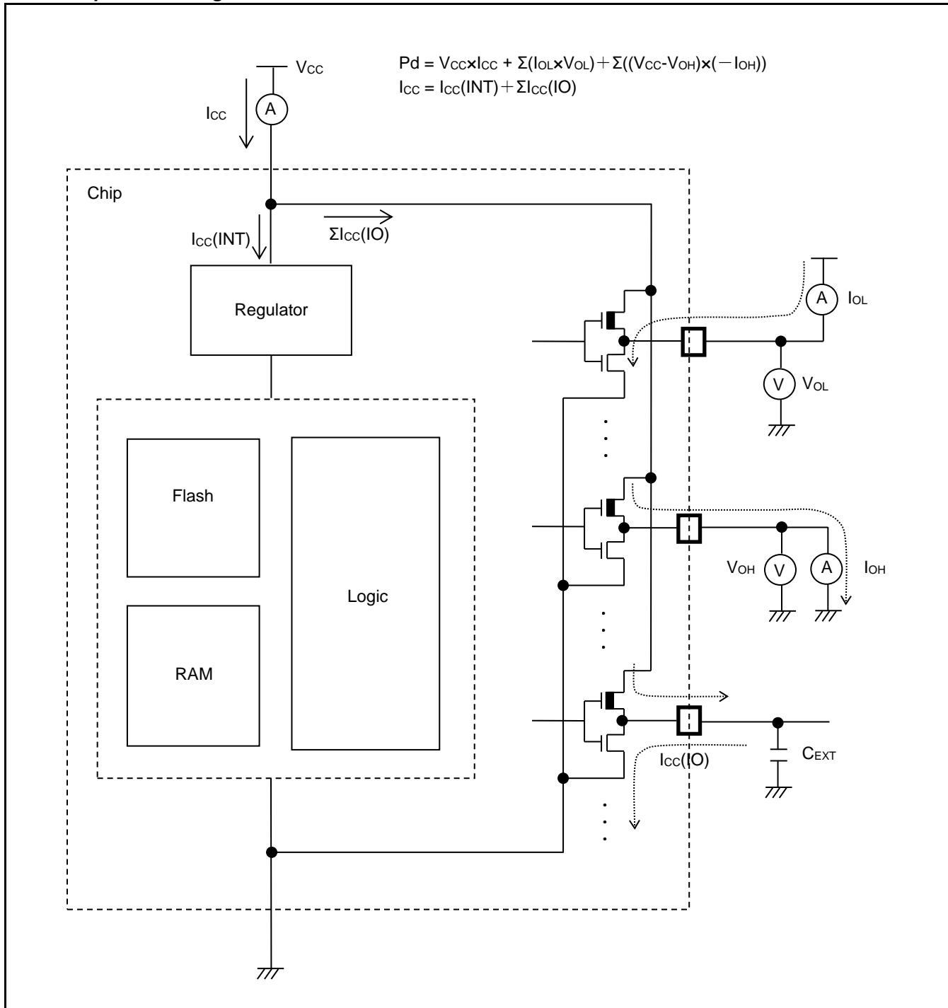
**Table 12-4 Typical and Maximum Current Consumption in Normal Operation(other than PLL), Code with Data Accessing Running from Flash Memory (Flash 0 wait-cycle Mode and Read Access 0 wait)**
