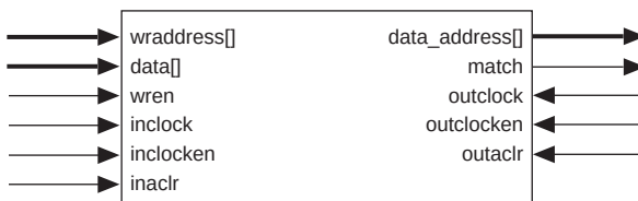
Figure 23. APEX 20KE CAM Block Diagram
