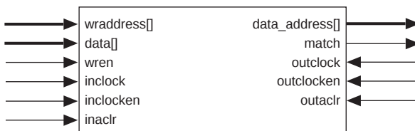
Figure 23. APEX 20KE CAM Block Diagram
