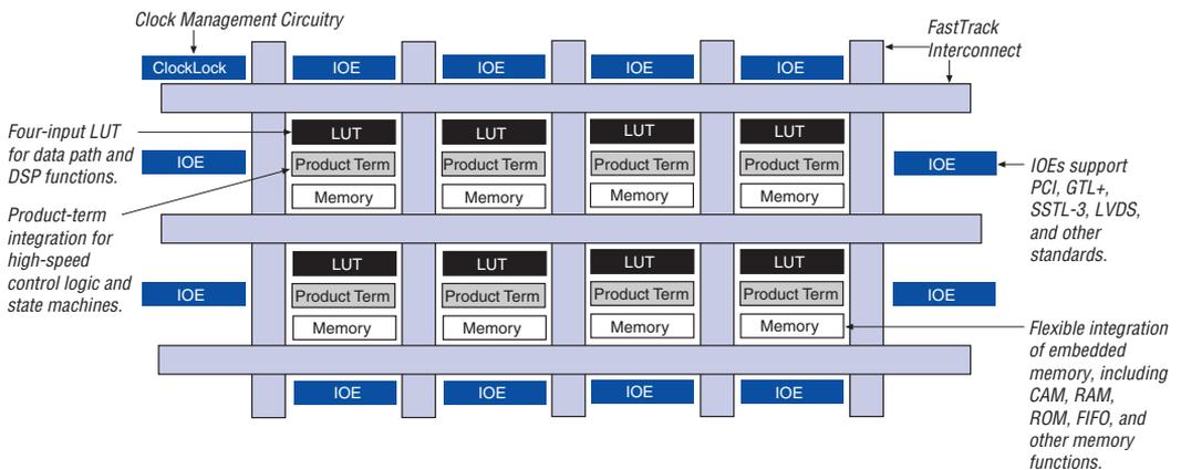
Each LE has two outputs that drive the local, MegaLAB, or FastTrack Interconnect routing structure. Each output can be driven independently by the LUT's or register's output. For example, the LUT can drive one output while the register drives the other output. This feature, called register packing, improves device utilization because the register and the LUT can be used for unrelated functions. The LE can also drive out registered and unregistered versions of the LUT output.
