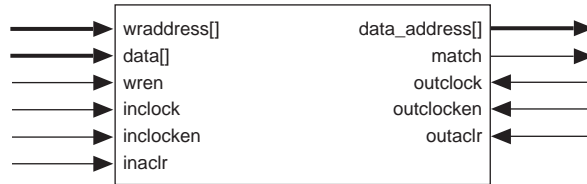
Figure 23. APEX 20KE CAM Block Diagram
