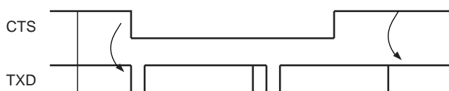
Figure 37-28. Transmitter Behavior when Operating with Hardware Handshaking
