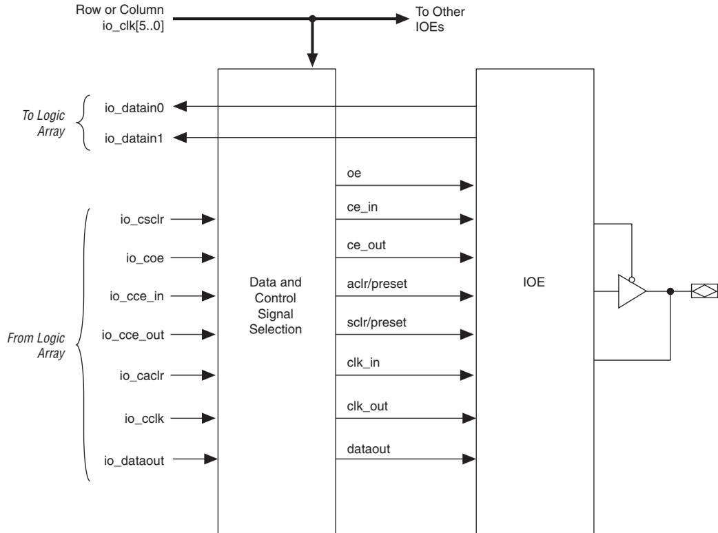
Each IOE contains its own control signal selection for the following control signals: `oe`, `ce_in`, `ce_out`, `aclr/preset`, `sclr/preset`, `clk_in`, and `clk_out`. Figure 2-24 illustrates the control signal selection.
