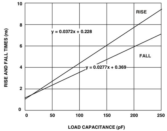
Figure 45. SDCLK Typical Output Rise/Fall Time
