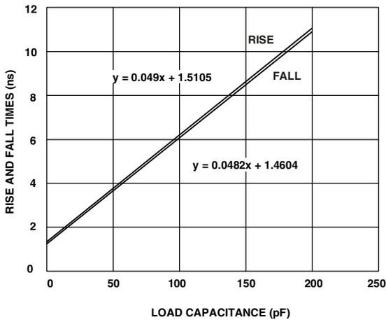
Figure 43. Typical Output Rise/Fall Time
