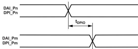
Figure 14. DAI/DPI Pin to Pin Direct Routing
