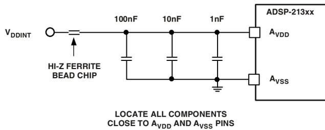
Figure 3. Analog Power ( $A_{VDD}$ ) Filter Circuit
