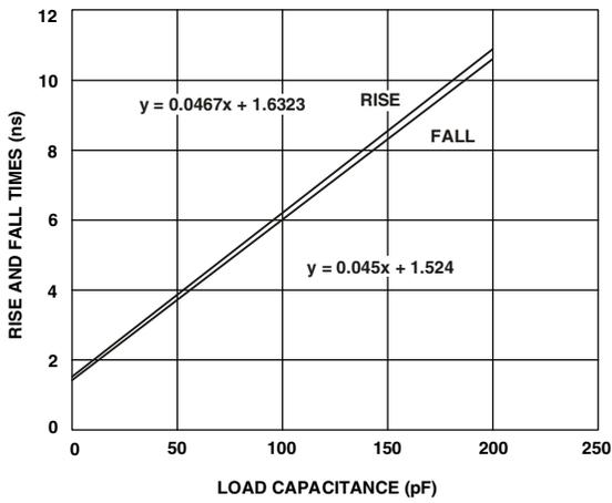
Figure 44. Typical Output Rise/Fall Time
