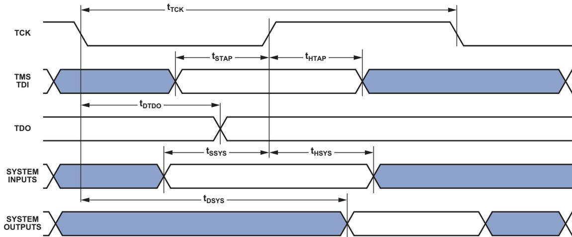
Figure 38. IEEE 1149.1 JTAG Test Access Port
