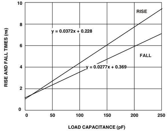
Figure 45. SDCLK Typical Output Rise/Fall Time
