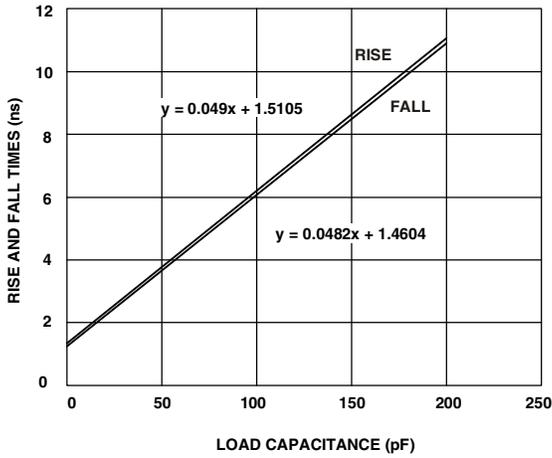
Figure 43. Typical Output Rise/Fall Time
