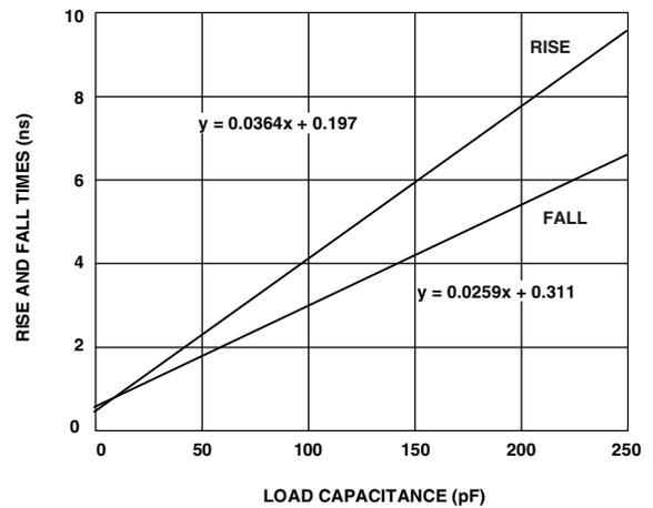
Figure 46. SDCLK Typical Output Rise/Fall Time
