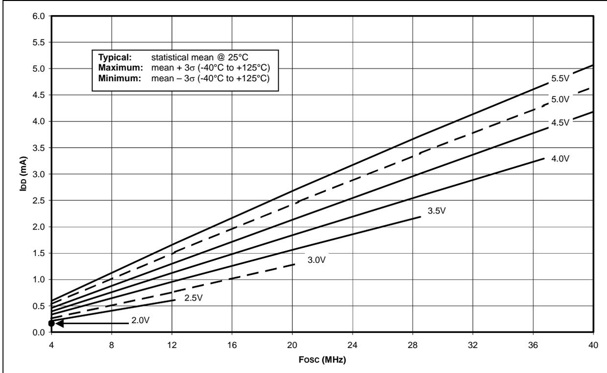
**FIGURE 23-23: TOTAL I<sub>PD</sub>, -40°C TO +125°C SLEEP MODE, ALL PERIPHERALS DISABLED**
