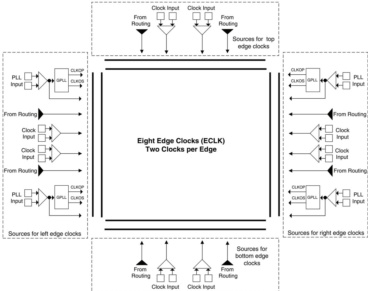
Note: This diagram shows sources for the LA-LatticeXP2-17 device. Smaller LA-LatticeXP2 devices have two GPLLs.
