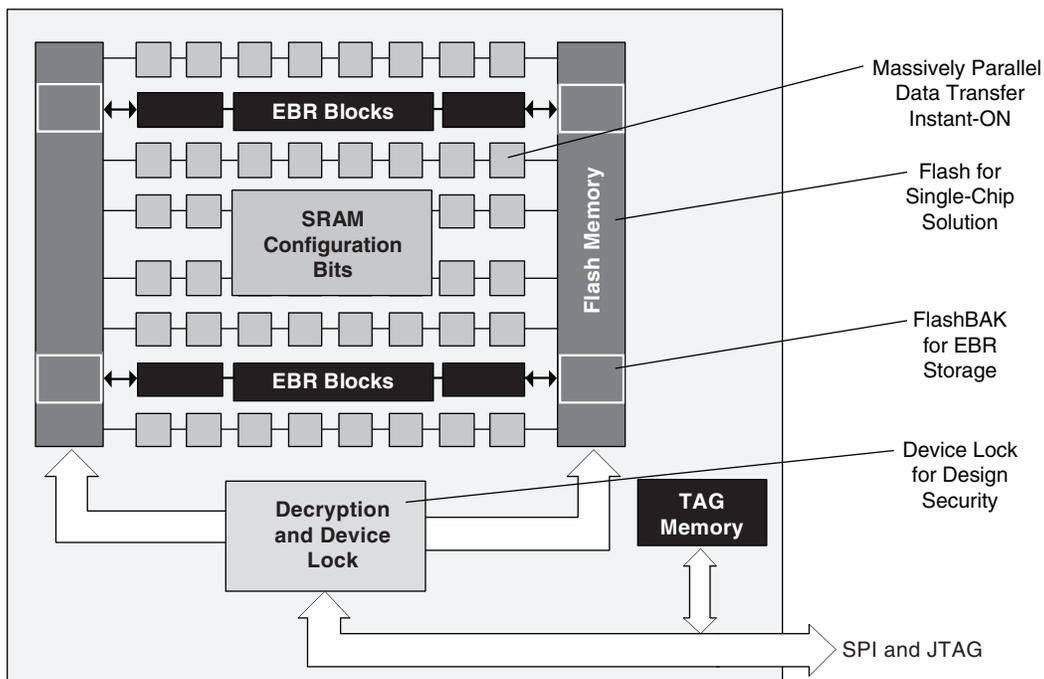
At power-up, or on user command, data is transferred from the on-chip Flash memory to the SRAM configuration cells that control the operation of the device. This is done with massively parallel buses enabling the parts to operate within microseconds of the power supplies reaching valid levels; this capability is referred to as Instant-On.
