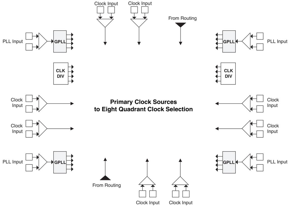
Note: This diagram shows sources for the LA-LatticeXP2-17 device. Smaller LA-LatticeXP2 devices have two GPLLs.
