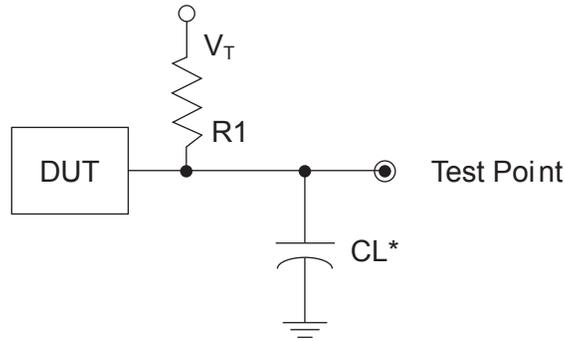
\*CL Includes Test Fixture and Probe Capacitance
