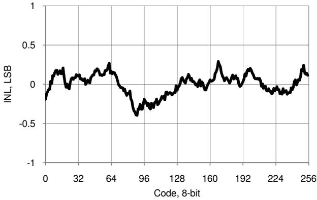
**Figure 11-41. IDAC INL vs Input Code, Range = 255  $\mu$ A, Sink Mode**
