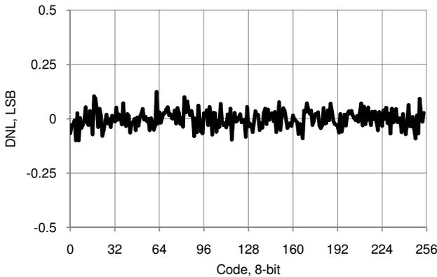
**Figure 11-43. IDAC DNL vs Input Code, Range = 255  $\mu$ A, Sink Mode**
