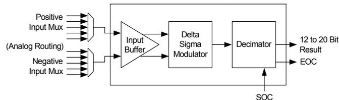
Resolution and sample rate are controlled by the Decimator. Data is pipelined in the decimator; the output is a function of the last four samples. When the input multiplexer is switched, the output data is not valid until after the fourth sample after the switch.
