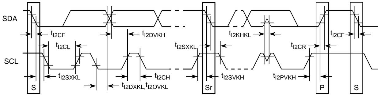
Figure 34. I<sup>2</sup>C Bus AC Timing Diagram
