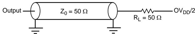
**Figure 29. AC Test Load for the JTAG Interface**
