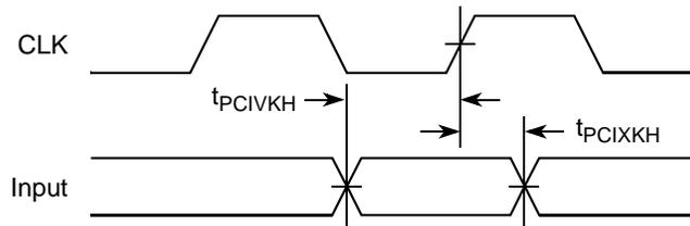
Figure 36. PCI/PCI-X Input AC Timing Measurement Conditions
