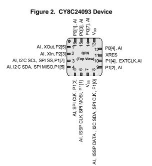
**LEGEND** A = Analog, I = Input, O = Output, OH = 5 mA High Output Drive, R = Regulated Output.
