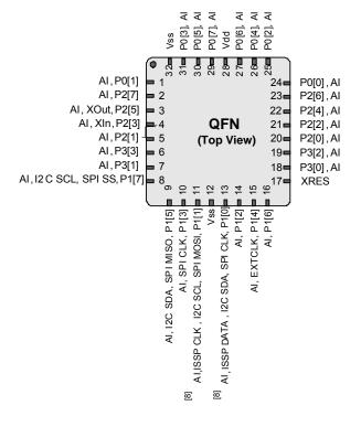
**LEGEND** A = Analog, I = Input, O = Output, OH = 5 mA High Output Drive, R = Regulated Output.
