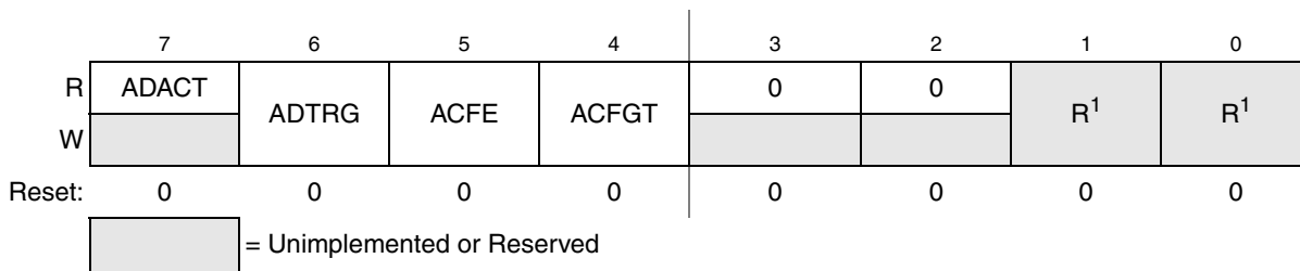
Figure 9-5. Status and Control Register 2 (ADCSC2)
