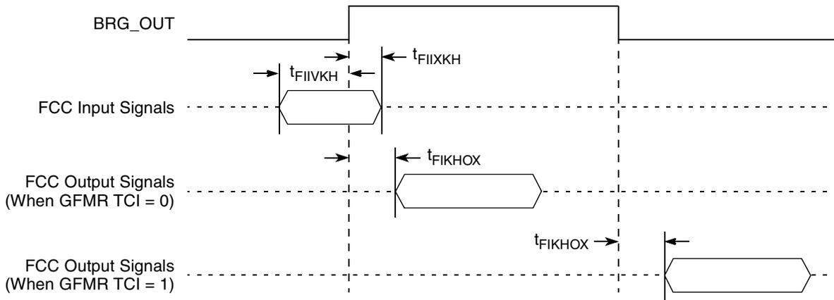
Figure 24. FCC Internal AC Timing Clock Diagram
