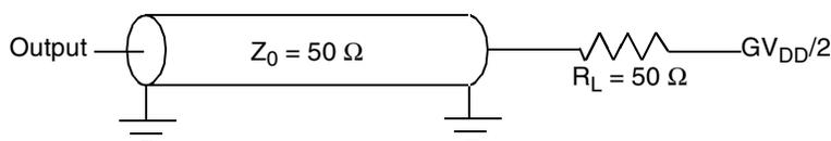
**Figure 5. DDR AC Test Load****Table 17. DDR SDRAM Measurement Conditions**
