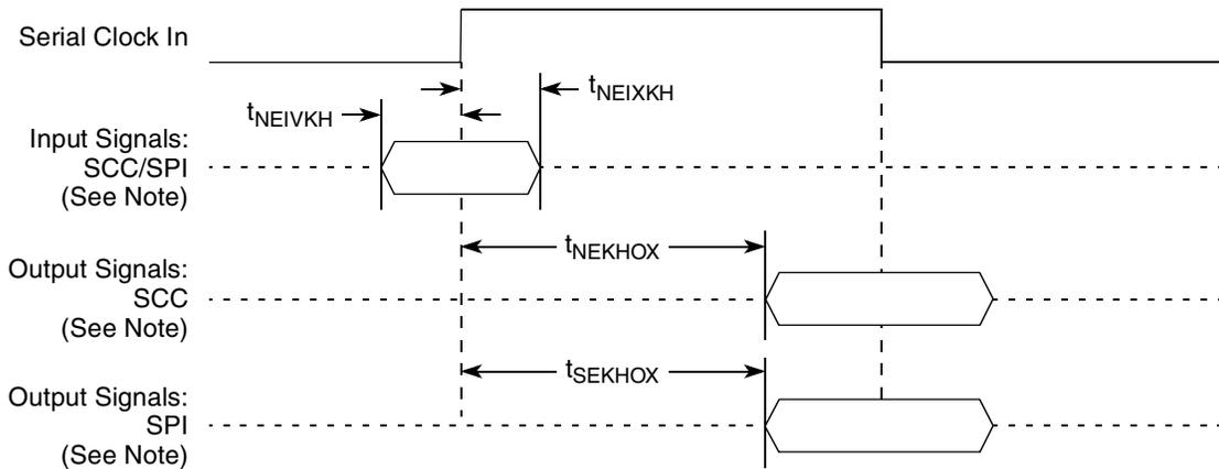
**Note:** The clock edge is selectable on SCC and SPI.
