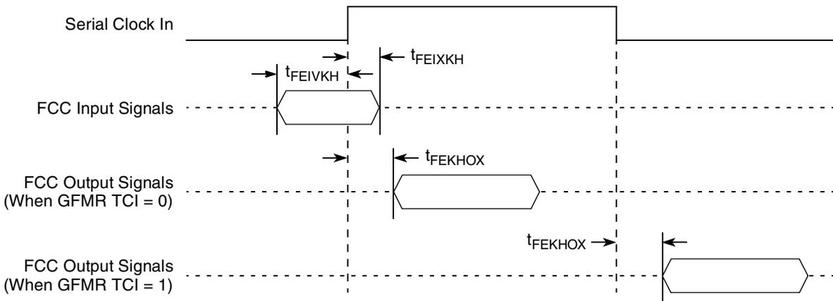
Figure 25. FCC External AC Timing Clock Diagram
