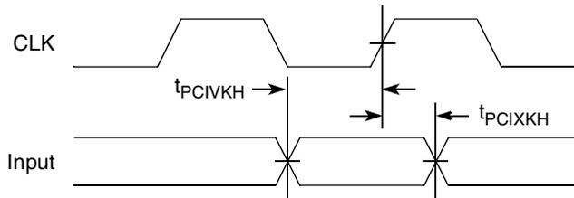
Figure 39. PCI-PCI-X Input AC Timing Measurement Conditions
