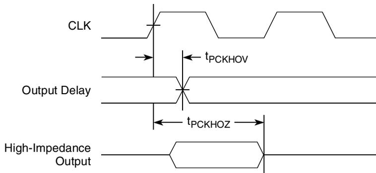
Figure 40. PCI-PCI-X Output AC Timing Measurement Condition
