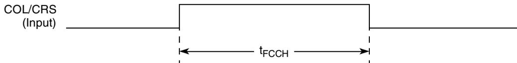
Figure 26. Ethernet Collision AC Timing Diagram (FCC)
