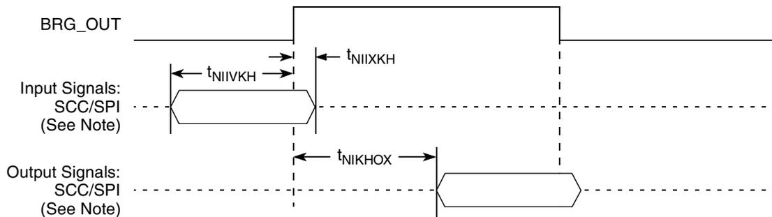
**Note:** The clock edge is selectable on SCC and SPI.
