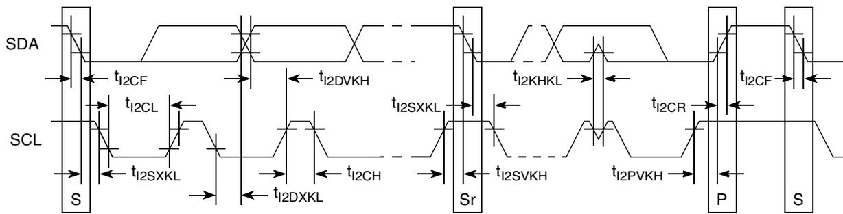
Figure 37. I<sup>2</sup>C Bus AC Timing Diagram
