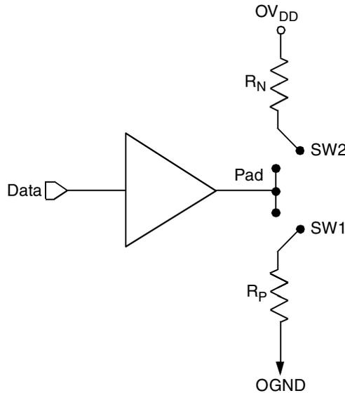
Figure 59. Driver Impedance Measurement
