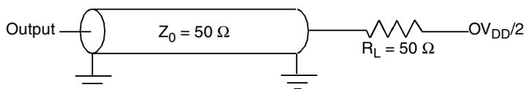
**Figure 36. I<sup>2</sup>C AC Test Load**
