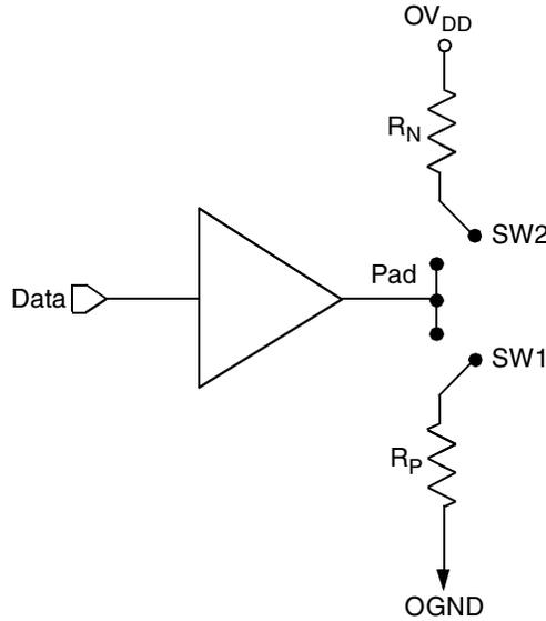
Figure 59. Driver Impedance Measurement
