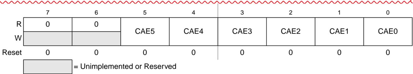
**Figure 10-7. PWM Center Align Enable Register (PWMCAE)**
