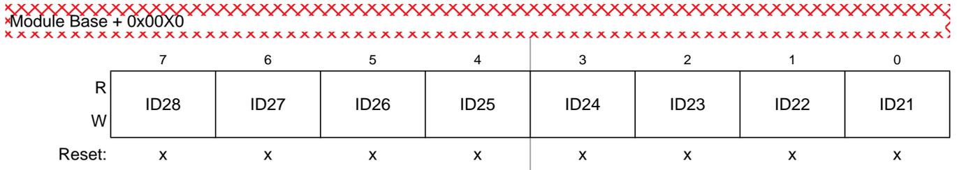
Figure 8-26. Identifier Register 0 (IDR0) — Extended Identifier Mapping
