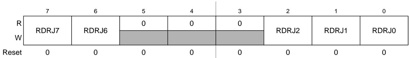
Figure 2-50. Port J Reduced Drive Register (RDRJ)
