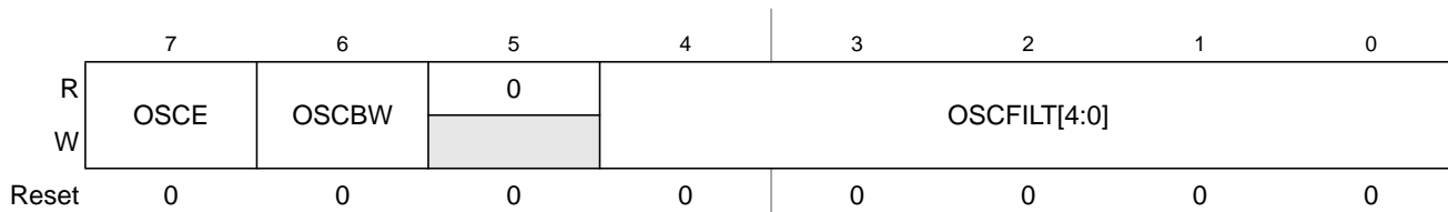
Figure 7-28. S12CPMU Oscillator Register (CPMUOSC)
