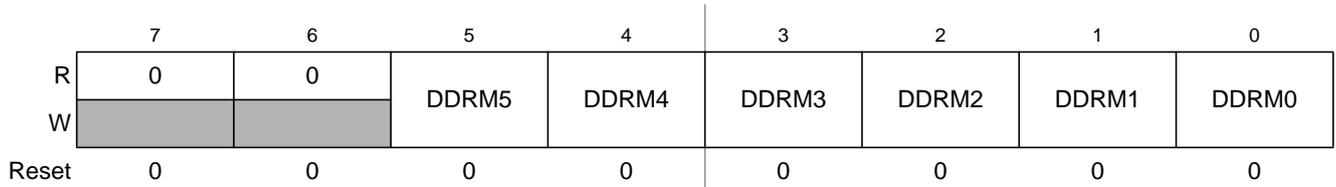
**Figure 2-32. Port M Data Direction Register (DDRM)**
