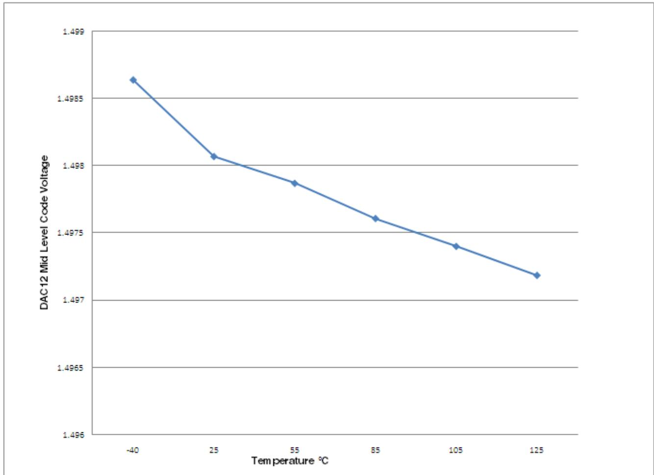
Figure 19. Offset at half scale vs. temperature
