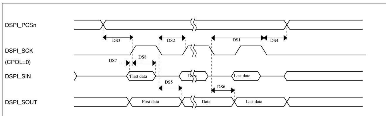
Figure 19. DSPI classic SPI timing — master mode
