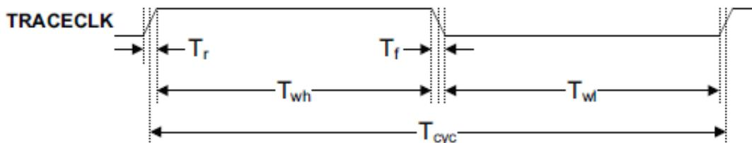
**Figure 3. TRACE\_CLKOUT specifications**
