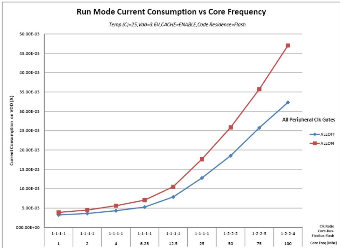
Figure 2. Run mode supply current vs. core frequency
