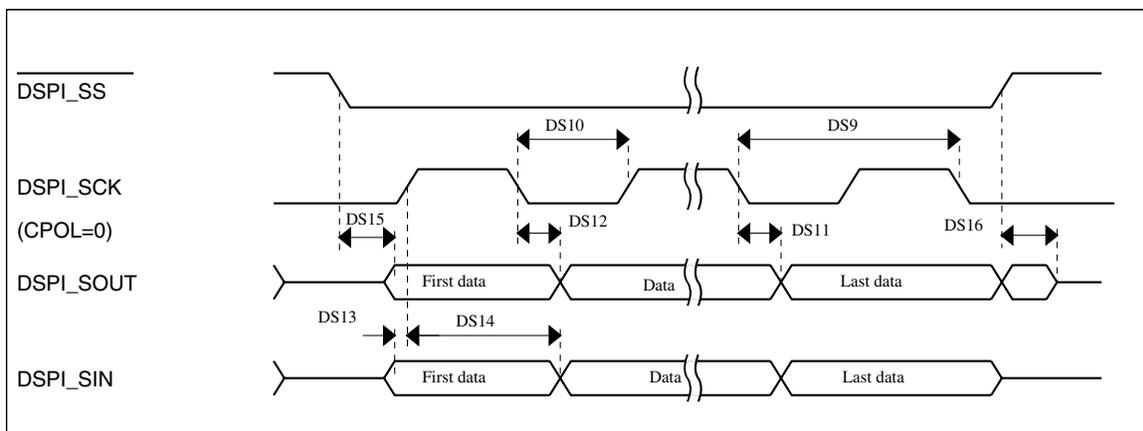
Figure 20. DSPI classic SPI timing — slave mode
