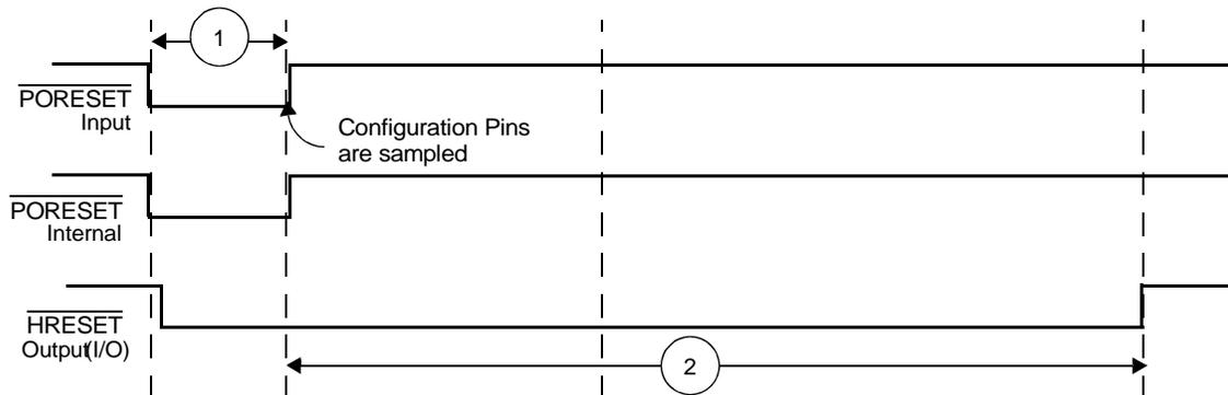
**Figure 4. Timing Diagram for a Reset Configuration Write**
