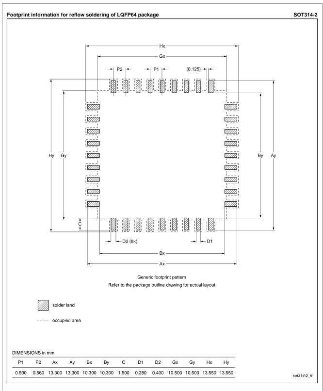
Fig 33. LQFP64 Soldering footprint
