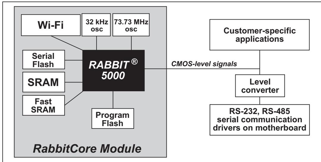
**Figure 6. RCM5400W Subsystems**
