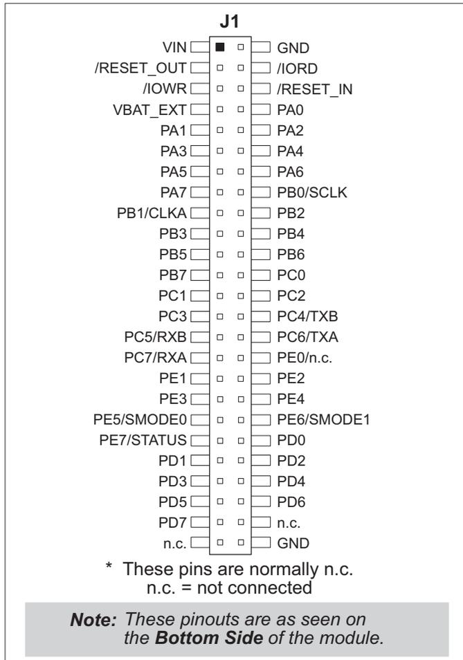
**Figure 7. RCM5400W Pinout**
