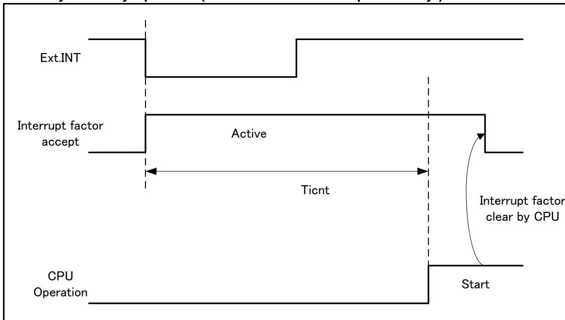
\*: External interrupt is set to detecting fall edge.
