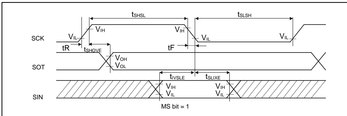
**Synchronous Serial (SPI = 1, SCINV = 1)**
