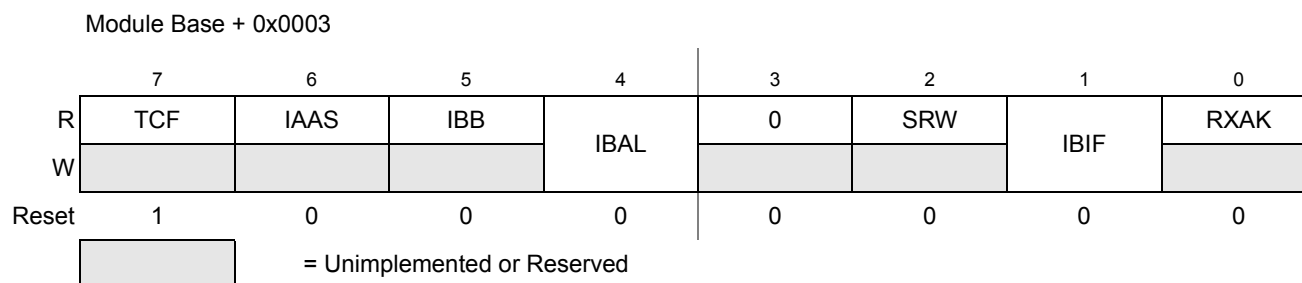
Figure 14-7. IIC Bus Status Register (IBSR)
