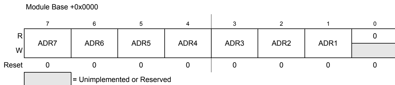
Figure 14-3. IIC Bus Address Register (IBAD)
