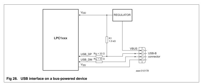
**Remark:** When a bus-powered circuit as shown in <u>Figure 28</u> is used, configure the <u>PIO0\_3/USB\_VBUS</u> pin for GPIO (PIO0\_3) in the IOCON block to ensure that the USB\_CONNECT signal can still be controlled by software. For details on the soft-connect feature, see the *LPC11U3x user manual* (Ref. 1).
