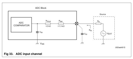
The effective input impedance, R<sub>in</sub>, seen by the external voltage source, V<sub>EXT</sub>, is the parallel impedance of ((1/f<sub>s</sub> x C<sub>ia</sub>) + R<sub>mux</sub> + R<sub>sw</sub>) and (1/f<sub>s</sub> x C<sub>io</sub>), and can be calculated using Equation 1 with
