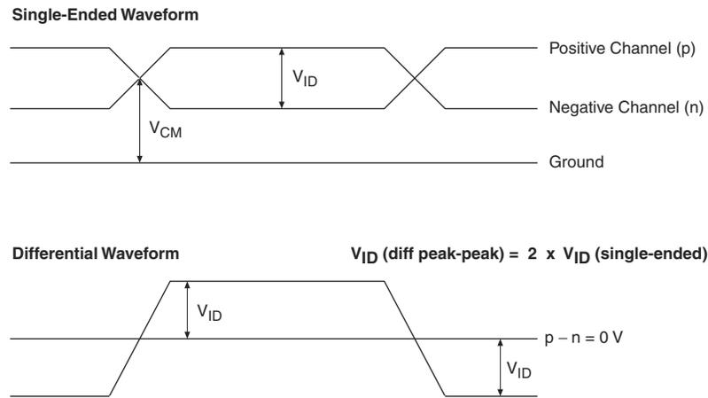
**Figure 4-4.** Transmitter Output Waveform
