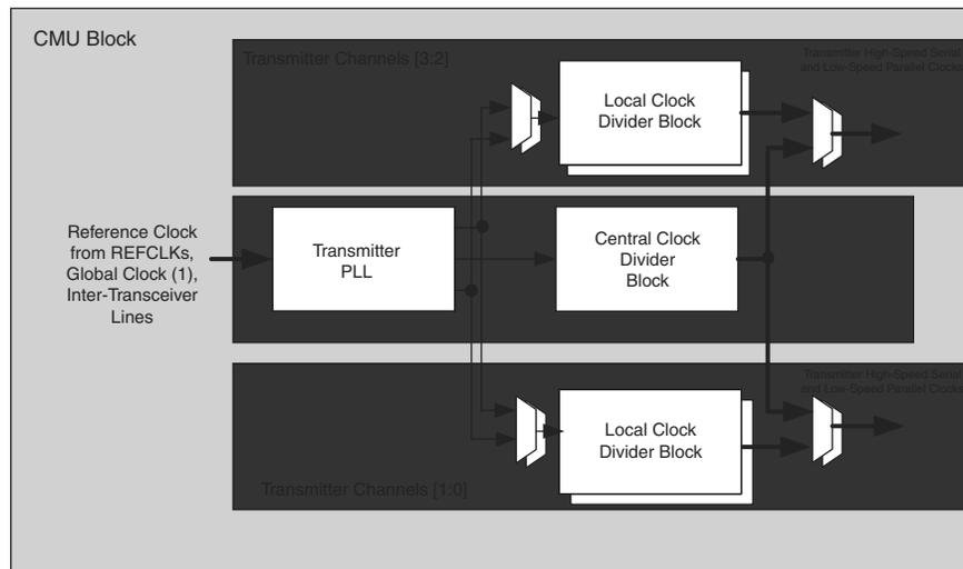
The transmitter PLL multiplies the input reference clock to generate the high-speed serial clock required to support the intended protocol. It implements a half-rate voltage controlled oscillator (VCO) that generates a clock at half the frequency of the serial data rate for which it is configured.
