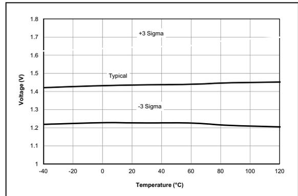
**FIGURE 38-24:** POR Rearm Voltage,  $V_{REGPM1} = 0$ , PIC16F18856/76 Only.
