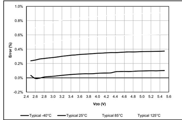
**FIGURE 38-76:** FVR Voltage Error 2x, PIC16F18856/76 Only.
