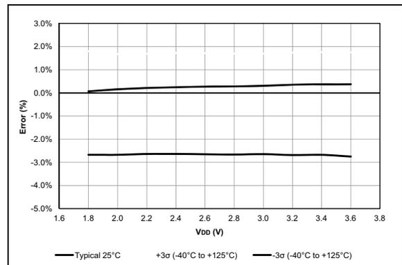
**FIGURE 38-78:** HFINTOSC Typical Frequency Error, PIC16LF18856/76 Only.
