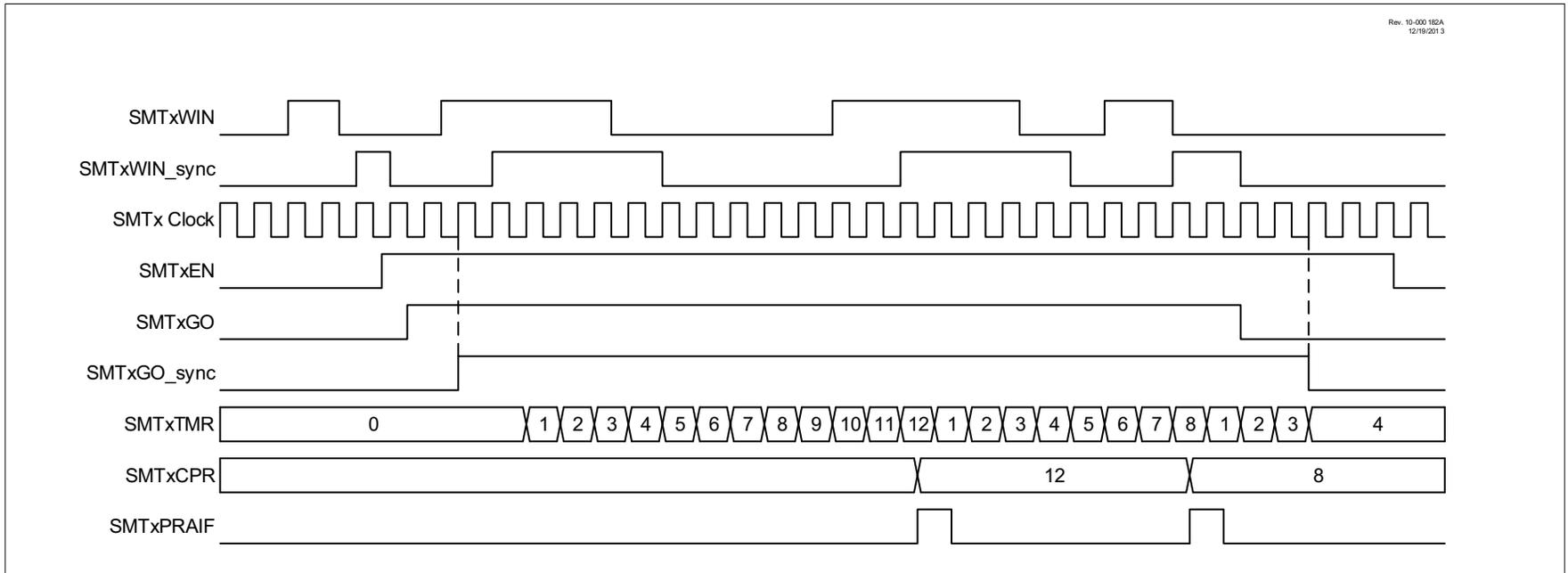
**FIGURE 32-22: WINDOWED COUNTER MODE SINGLE ACQUISITION TIMING DIAGRAM**
