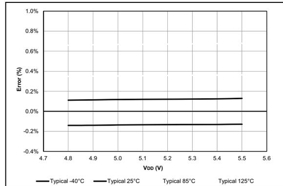
**FIGURE 38-77:** FVR Voltage Error 4x, PIC16F18856/76 Only.
